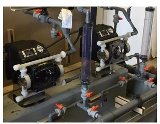
When the MD3's first diaphragm is in the suction phase, the second diaphragm is in the discharge phase. This causes gaseous fluids to be pumped through the without causing vapor lock.
